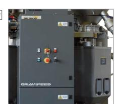
Continuous gravimetric blender, designed to blend pellets, regrind and flakes in extrusion processes where key-factors are the dosing accuracy and the capability to follow and compensate the variations of unstable processes.
